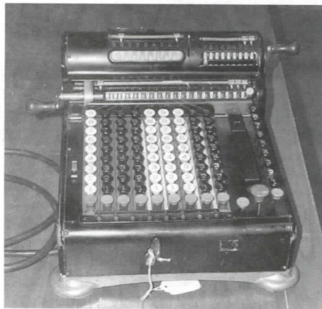
1923 Marchant Model EEG9 electric pinwheel calculating machine loaned to PBS by the Historical Museum at St. Gertrude. [Photo courtesy of the Historical Museum at St. Gertrude]
